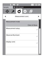
2 Use [▲] or [▼] to move the cursor to the desired measurement mode.
