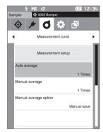
3 After setting the measurement conditions, press the [ESC] button to return to the previous screen.
