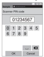
3 After inputting the numbers, move the cursor to [OK] and press the [Confirmation] key.
