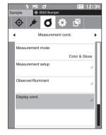
2 Use [▲] or [▼] to move the cursor to "Display cond.", and then press the [Confirmation] key. The <Display cond.> screen is displayed.
