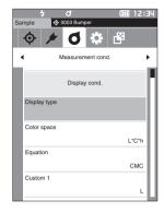
2 Use [▲] or [▼] to move the cursor to the desired display type, and then press the [Confirmation] key.
