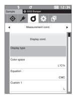
3 After setting the display conditions, press [ESC] to return to the previous screen.
