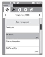
2 Use [▲] or [▼] to move to the cursor to the group number column to which the current target color should be applied, and then press the [Confirmation] key.
